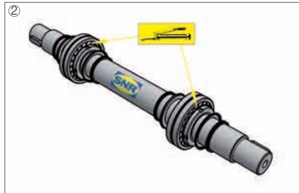
② Clamp the shaft horizontally (protect the shaft against damage in the area of the clamping). The internal contact washers and V-rings are slid onto the shaft first. The sequence and arrangement of the sealing elements is crucial to ensure correct mounting.
